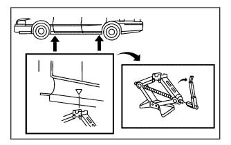
For all wheel types, find the jacking location using the diagram above and the corresponding hoisting notches located on the bottom side of the plastic molding. The notches in the plastic molding are marked with a triangle shape to help you find them.
